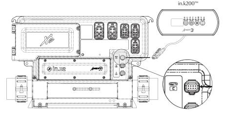
Connect the main keypad in.k200<sup>™</sup> as indicated here.
