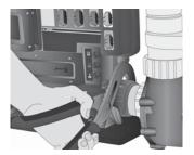
Unplug all LC (Low Current) outputs. e.g.: main keypad, light or any other accessory. Disconnect the grounding cable from the Bonding Lug of the in.xe<sup>™</sup> Spa Pack.
