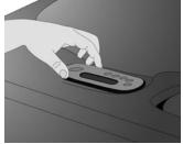
With an scraper tool, gently clean the surface of installation of the new keypad, finish the job with an alcohol saturated paper towel to remove any unwanted residue left over from the old keypad. Feed the cable of the new keypad through the hole opening in the spa.
