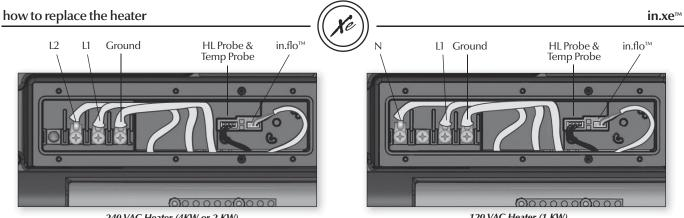
240 VAC Heater (4KW or 2 KW)
