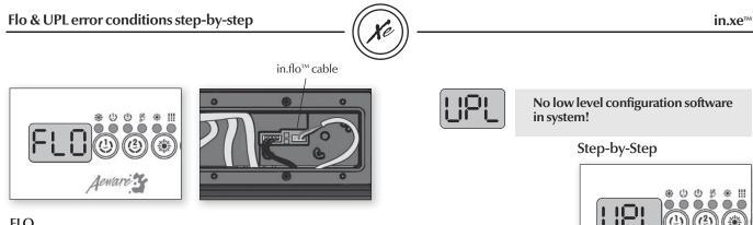
FLO Primary pump is activated but the system doesn't detect any water flow
