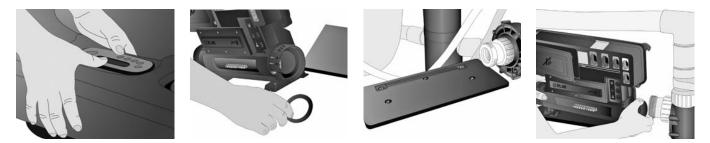
Secure the keypad in place. Insure that its adhesive strip is properly glued by pressing evenly with your finger over the entire surface. Place a rubber 2" O'ring gasket at the end of each heater nut, to prevent water leakage between the heater nuts and the 2" PVC heater tailpieces. When installing the new in.xe<sup>™</sup> spa pack, slide back side of the unit's feet into the guide plate.
